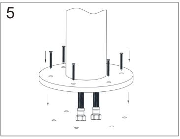
5. Fix the base on the ground by screws.
