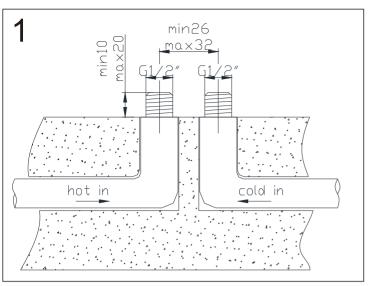
1. Pre-bury the water pipes under the ground, hot in (left), cold in (right).
