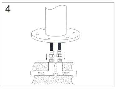
4. Screw the hoses to the connectors of the water pipes.
