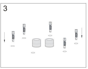
3. Put the drywall anchors in the holes drilled.
