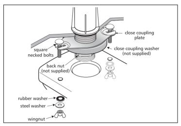
Push close coupling washer onto back nut, this ensures centralisation before offering up to closet.
