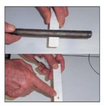
The adjustable strip is essential for the operation. Take the mid-point of the stick as base point. Apply the gap dimension symmetrically on the strip. Cut off the overage on the strip, for both ends.
