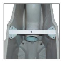
Place the main mounts on the strip. Check the gap now with trip; mounts on it. The length of the strip may neither long nor short.
