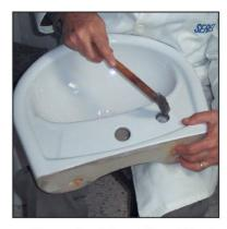
The central tap holes are left open during the mass production. For recessed tap systems; the closed holes at left and right sides must be open with a sharp pointed hammer with patience, from the top.
